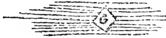
FIG. 26.—Cube of galena, G, replacing limestone. The crystal squarely intersects the shaley layers. Drawn by the writer from specimen from mines of Federal Lead Co., Mo.
